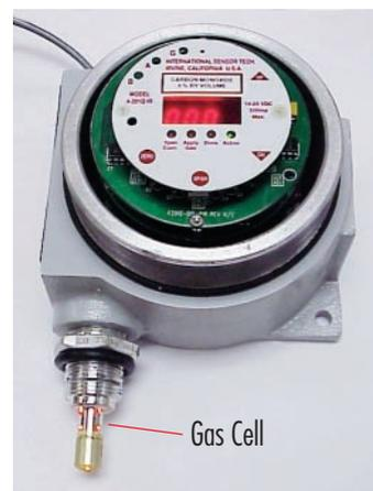
*Fig. 1 An example of an IR gas monitor with the gas cell assembly exposed.*
