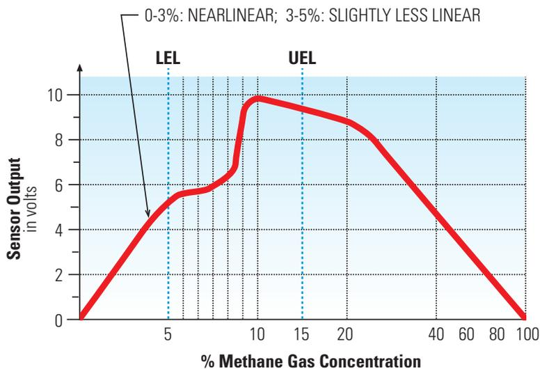
Fig. 5 Sensor Output vs. Gas Concentration
