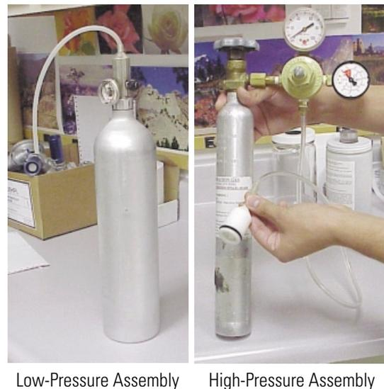
Fig. 2 Calibration Gas Bottles
